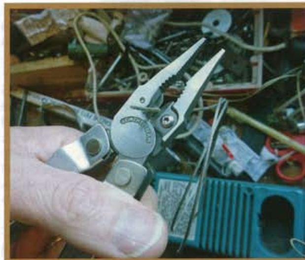
The wire cutters are toughened and the blades are replaceable. Handy not just for around your campsite but also for so many jobs around the home.
